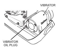
Figure 10. Vibrator Oil Plug
